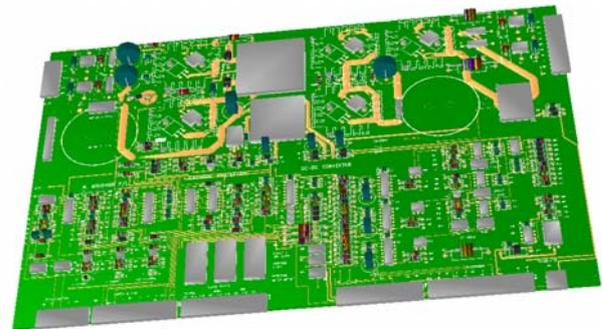
View of D5625 DC/DC Converter system. The single circuit board contains an isolated converter, surge suppression, status leds and relays, interruptor relay and transducer interface outputs.
